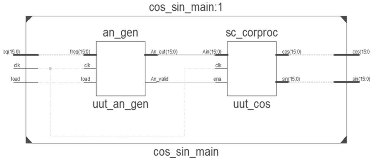
Figure 5. Sinusoids generator architecture
