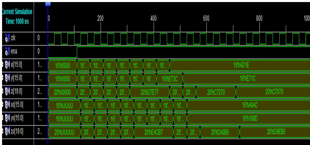
Figure 10. Simulation results of pipeline CORDIC algorithm in one stage
