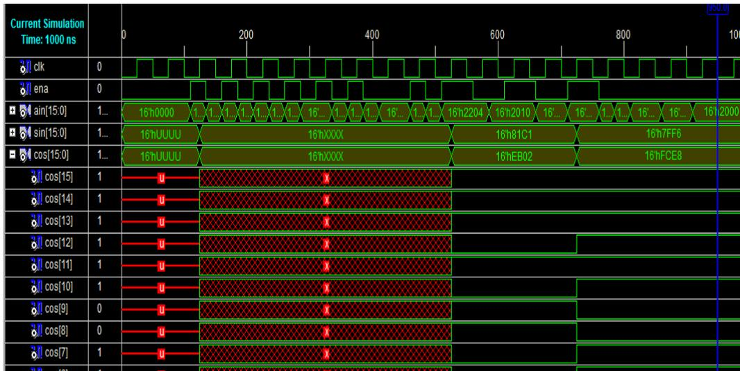
Figure 8. Simulation results of pipeline CORDIC 8 stages
