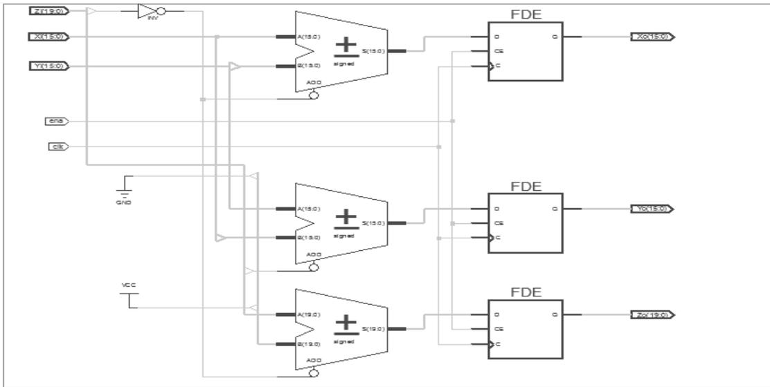
Figure 9. The implementation of a pipelined CORDIC 1 stage
