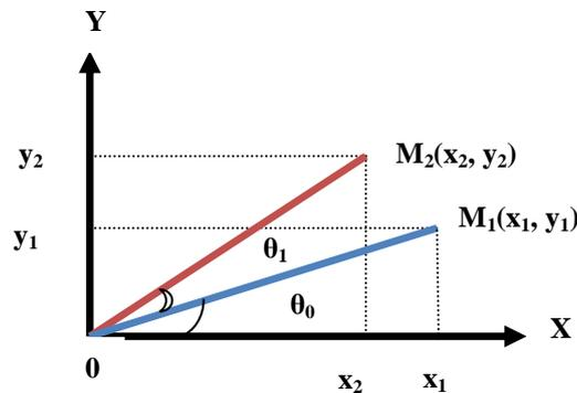
Figure 6. Decomposition of angle  $\theta$  in several micro-rotations
