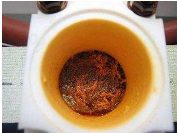
Figure 11. GFRP specimen after corrosion test with bromine.
