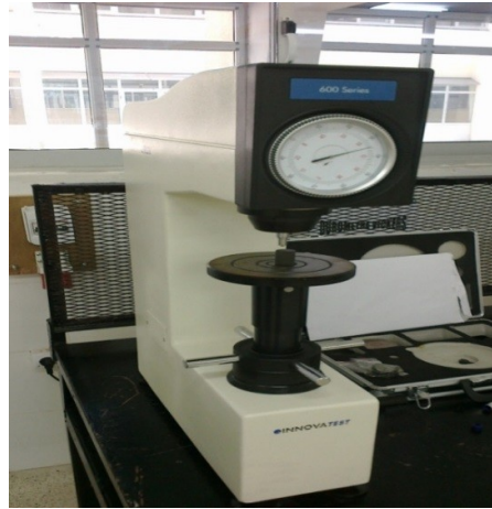
Figure 5: Apparatus used for the classic measure of the hardness
