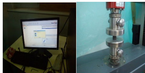
Figure 7: Compressive test device in cylinder sample tests
