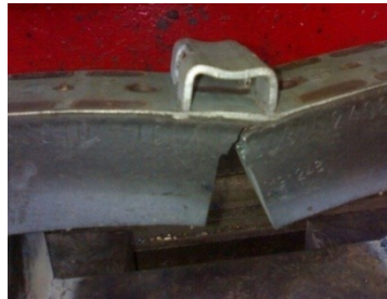
Figure 27: Result of the Type 1 flexural test
