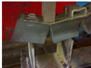
Figure 28: Result of the type2 test of flexion
