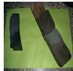
Figure 22: Take-off of the composite at the ends
