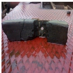
Figure 22: Take-off of the composite at the ends
